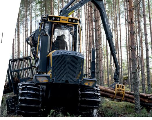
ETC is an intelligent system which means that it is self learing and therefore adapts and develops itself as you use it. Thanks to the function of the sensor's, you gain a smoother and more precise crane movement and position. The placement of the sensor's in the crane generates a robust and reliable system where maintainance is conducted in a smooth and easy way.
